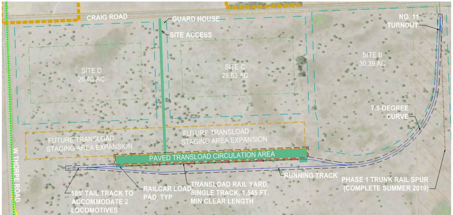
Figure 1-4 Phase 2 - Rail-Truck Transload Facility Design
