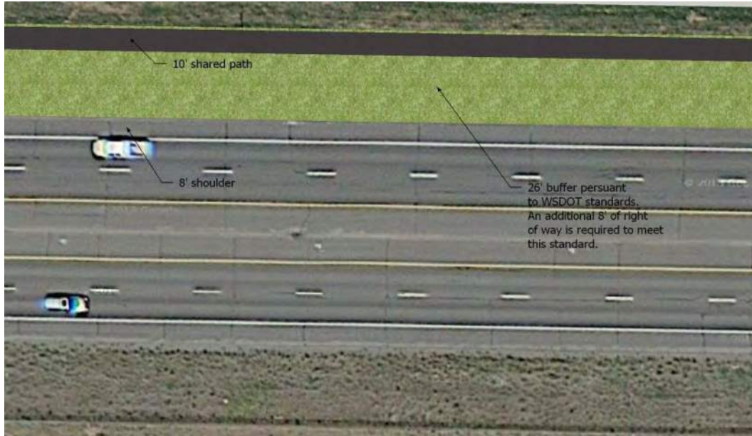
Figure 3-N Shared use path on the north side of US 2 between Mitchell Drive and Craig Road
