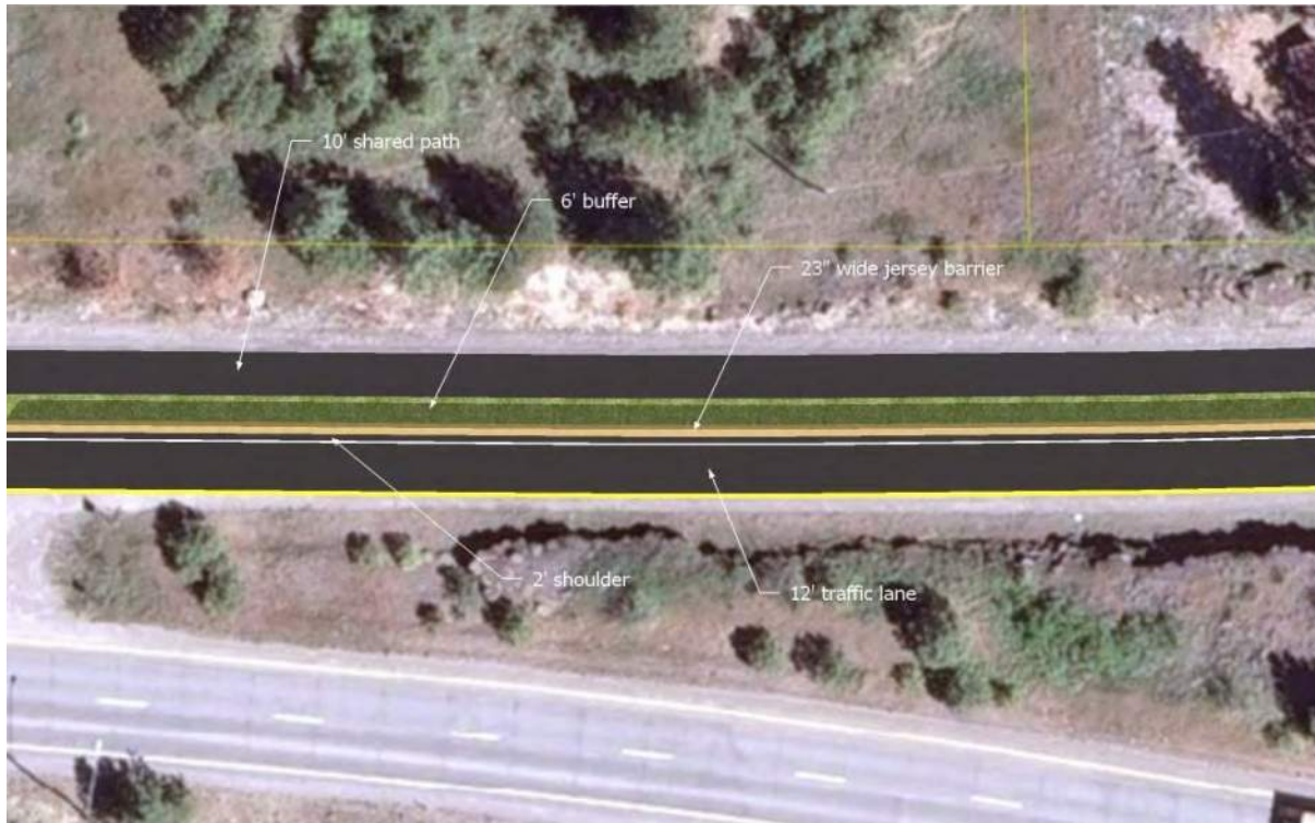
Figure 3-V West Plains Trail with a narrow buffer and a jersey barrier
