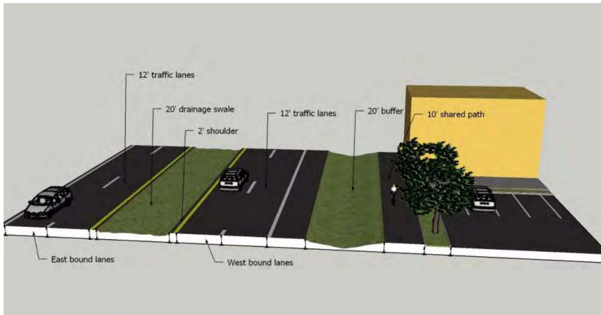
Figure 3-T Cross section concept of shared use path between Deer Heights and Spotted Road with a 30' setback
