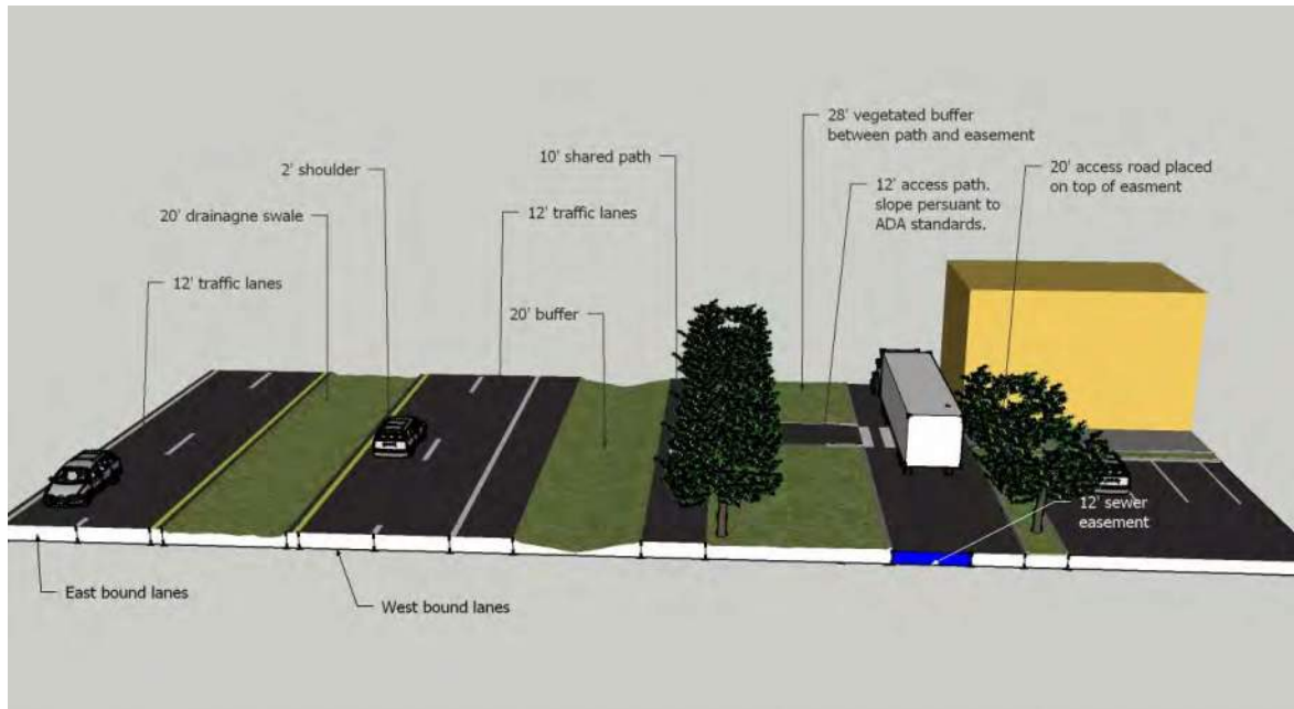
Figure 3-S Cross section concept of a shared use path between Deer Heights and Spotted Road with a 78' setback
