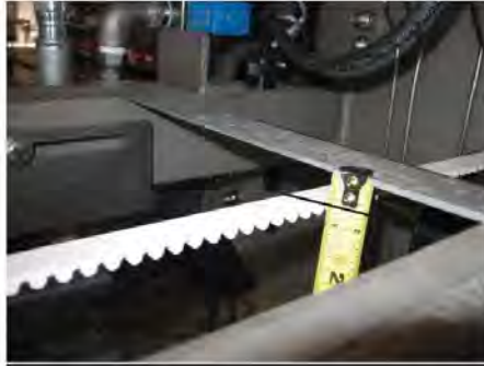
Figure 6-6. Trolley drive belt at idle end
