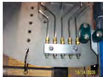
Figure 6-22. Carriage Roller Grease Fittings (Drivers Side)
